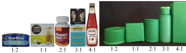
Fig. 3: Target objects spanning a variety of aspect ratios (noted below each object) used in simulation testing (left) and in physical experiments (right).
