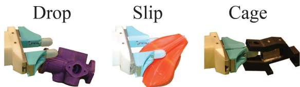
Fig. 6: Success and failures were hand labeled and fell into several categories. A drop failure occurred when the gripper failed to hold the object. A slip occurred when the gripper could not resist gravitational torque and rotated 10 degrees below horizontal. A cage failure occurred when the lift was successful despite positional errors.
