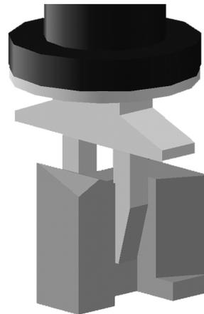
FIG 2. Computed Grip for Parallel-Jaw Gripper.
