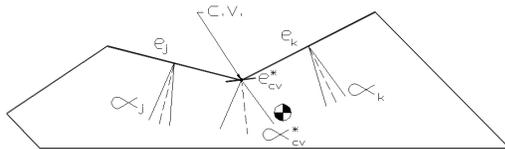
FIG 4. Edge  $e_{cv}^*$  and the friction cone at a convex vertex.
