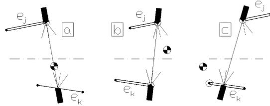
FIG 13. Some examples of minimum  $\delta$  grips. *a* has  $\delta = 0$ , *b* has  $\delta = \min$ , and *c* has  $\delta = \min$  after being perturbed to be within the friction cones.
