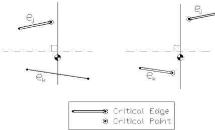
FIG 11. Critical Edges and Critical Points.
