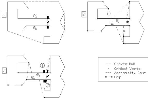
FIG 14. The steps for generating accessibility cones and modifying grips. a: Finding the convex hull of the part when a grip is inaccessible; b: Determining the critical vertices and accessibility cones; c: Creating the modified accessibility cones, and modifying the grips to [1]accessible minimum  $\phi$  grip, and [2]accessible minimum  $\delta$ ) grip.
