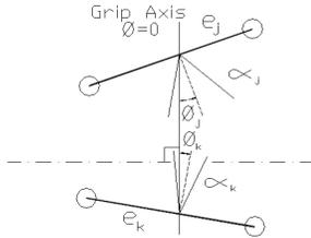
FIG 6. When  $\phi=0$  frictional dependence between the two edges is balanced.
