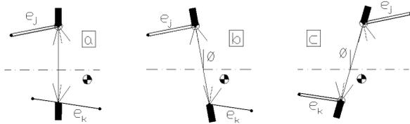
FIG 12. Some examples of minimum  $\phi$  grips. *a* has  $\phi = 0$  while *b* and *c* have  $\phi = \min$ .
