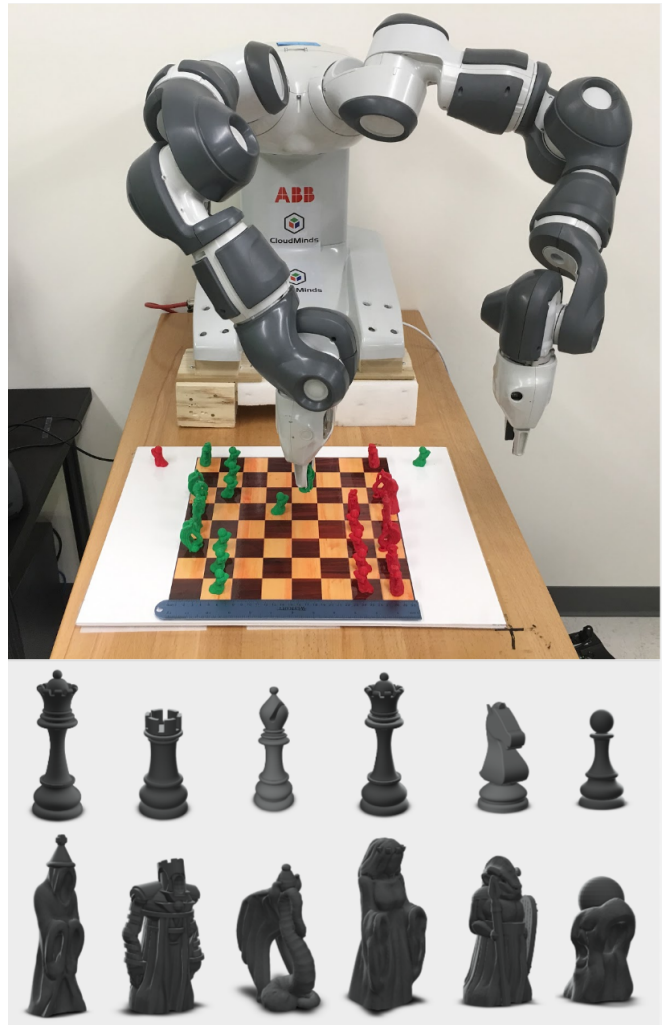
Fig. 2. (Top) The YuMi robot replaying the classic 1997 chess game where IBM’s Deep Blue defeated world champion Garry Kasparov. (Bottom) CAD model renderings of standard chess pieces and the equivalent non-standard “Wizard” pieces.
