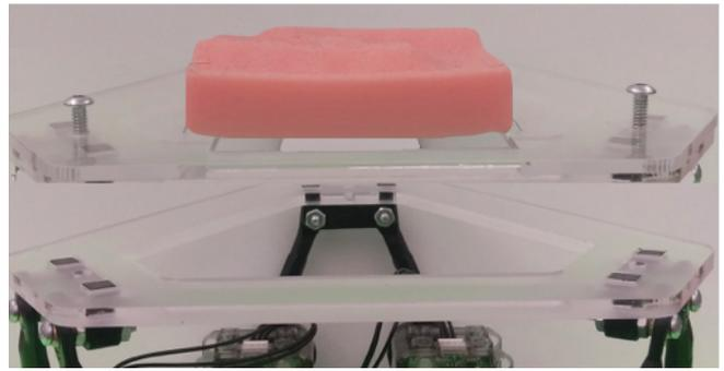
Fig. 3: The platform is modular with a removable top mount which allows for mounting tissue phantoms to create configurable FLS task environments.
