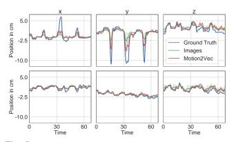
Fig. 5: Pose imitation on da Vinci robot arms from the Motion2Vec embedded video sequences using a feedforward neural network for left arm on *(top)* and right arm on *(bottom)* in comparison to ground-truth and image decoded poses. Results suggest 0.94 centimeter error in position per observation on the evaluation set. Ground-truth in blue, raw videos in green, predicted in red.
