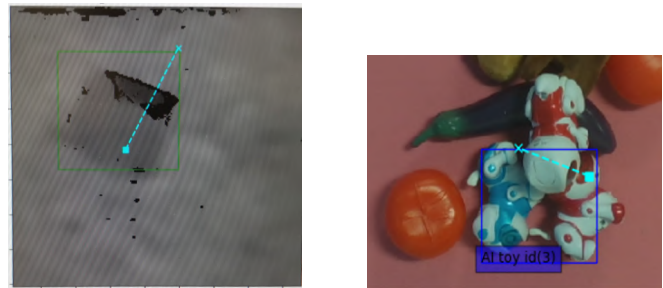
(a) FC-GQ-CNN computes a grasp on bulge that is caused by missing information in the depth image.
