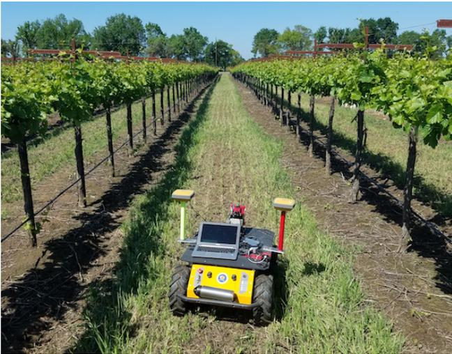
Fig. 1: A test platform for identifying challenges in navigation within a vineyard. Irrigation lines and vine stocks block travel between rows, thus creating motion constraints.
