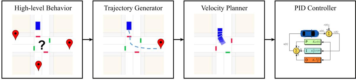
Fig. 4: The planner for the algorithmic supervisor. First, a high-level destination, specified as a destination lane, is randomly selected for the agent. Then a positional trajectory is generated via OMPL to take the agent to the goal position. A velocity planner is then called to ensure the agent reaches the destination without collisions or violation of traffic laws with respect to the traffic light. Finally, a PID controller is used to execute the planned path.
