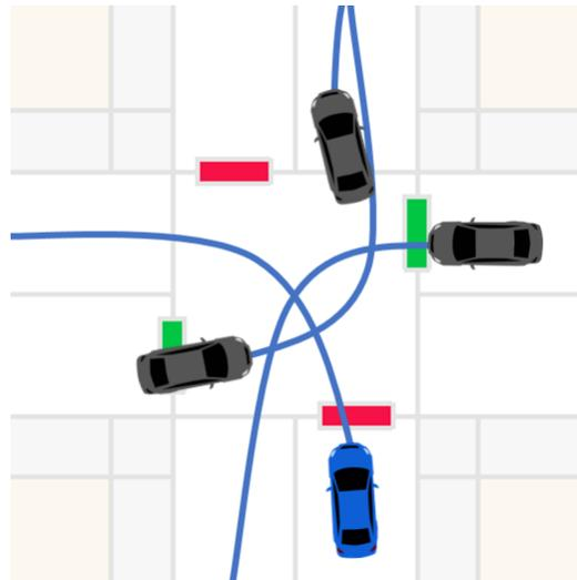
Fig. 1: An example of a driving intersection in FLUIDS showing four cars and traffic lights. FLUIDS focuses on efficiently modeling the interaction between different drivers and pedestrians. The colored lines represent paths generated by FLUIDS with collision-free velocities.
