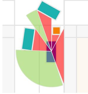
Fig. 5: Illustration of the quasi-LIDAR perspective state space. Rays are projected into the scene from the car's perspective. The red rays correspond to detected objects in the environment. The density of projected rays and noise model are both configurable.
