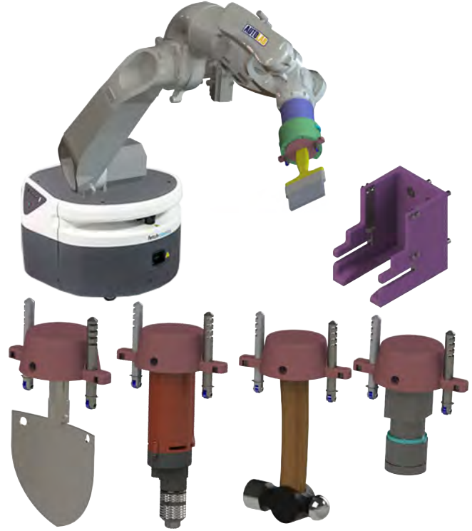
Fig. 1: Top: mobile manipulator robot equipped with the tool changer system, and tool housing. Bottom: example tools.
