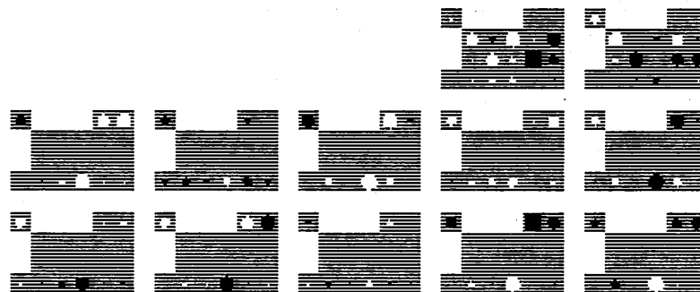
Figure 6-1: This network was trained on 298 samples taken uniformly from the state space of a simulated arm. The inputs (from left to right) are the position, velocity and desired acceleration of the shoulder joint and the position, velocity and desired acceleration of the elbow joint. The magnitude of the largest weight is 9.63.
