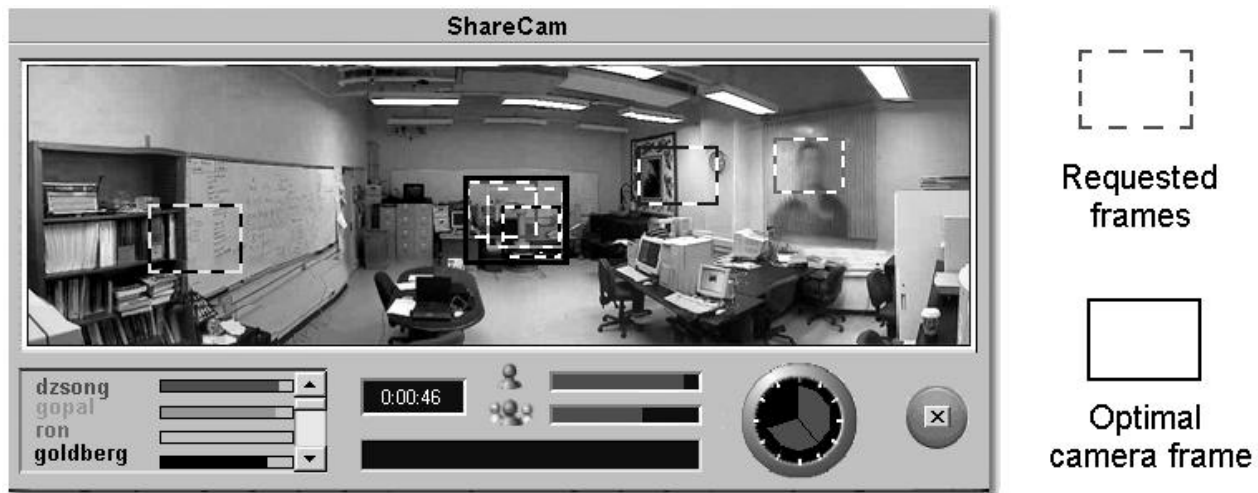
Figure 2: This figure illustrates ShareCam's Java-based user interface, which currently runs on most Windows based PCs. Users view two windows. One (not shown) displays a live video stream as captured by the robotic camera. The second window, illustrated here, contains the user interface. The panoramic image is a fixed photo of the camera's reachable range of view. The snapshot above shows 4 active users listed in the scrollable window at the left. Each user requests a camera frame by positioning a dashed rectangle over the panoramic image. Based on these requests, the algorithm computes an optimal camera frame (shown with solid rectangle), and serves the camera accordingly to displays the resulting live video stream. The horizontal bars indicate levels of user satisfaction as described below. The system is installed in our research lab at Berkeley but will be moved outdoors in April 2003.
