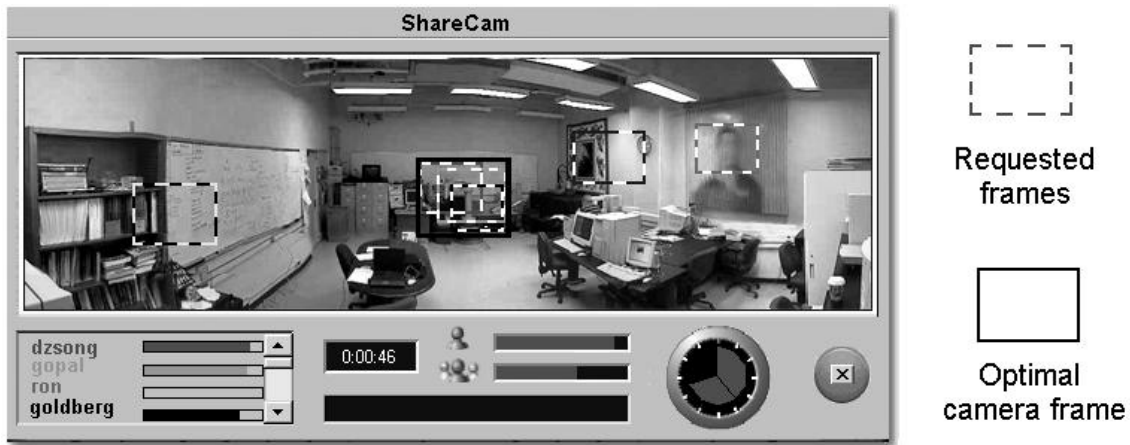
Fig. 2. This figure illustrates ShareCam's Java-based user interface, which currently runs on most Windows based PCs. Users view two windows. One (not shown) displays a live video stream as captured by the robotic camera. The second window, illustrated here, contains the user interface. The panoramic image is a fixed photo of the camera's reachable range of view. The snapshot above shows 4 active users listed in the scrollable window at the left. Each user requests a camera frame by positioning a dashed rectangle over the panoramic image. Based on these requests, the algorithm computes an optimal camera frame (shown with solid rectangle), and servoes the camera accordingly to displays the resulting live video stream. The horizontal bars indicate levels of user satisfaction as described below. The system is installed in our research lab at Berkeley but will be moved outdoors in April 2003.
