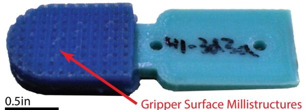
Fig. 1: **Top:** Grasp robustness for 37 gripper surfaces was evaluated using a 4-dof robot with a custom “reset” mechanism that includes an activated rewind mechanism and cable that lifts and replaces the object onto the worksurface in an upright position after each grasp. **Bottom:** Each gripper surface was cast in silicone polymer using custom 3D-printed molds.
