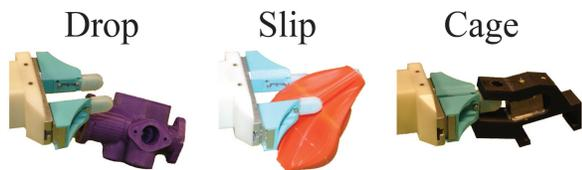
Fig. 6: Examples of the three failure cases.
