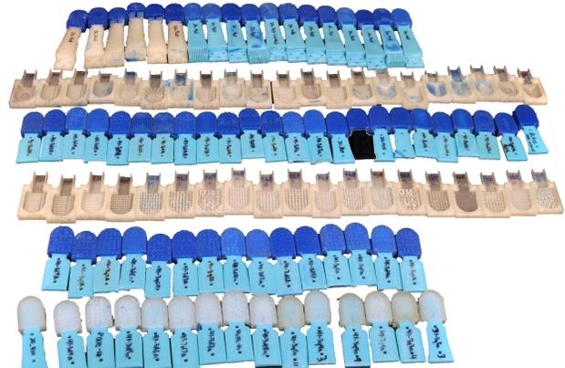
Fig. 2: The 37 gripper surface designs, with 3D printed molds (in white) used for fabrication.
