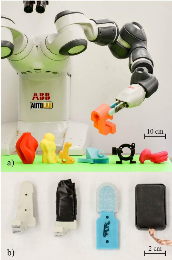
Fig. 9: (above) After the gripper tip surface design process, an ABB Yumi industrial robot was used to compare four gripper tip surfaces using a test set of eight objects: 80 trials for each gripper tip surface. (below) The four gripper tip surfaces from left to right: ABB default grippers, ABB grippers wrapped with electrical tape, the silicone design described above, and the gecko-inspired tip surfaces.
