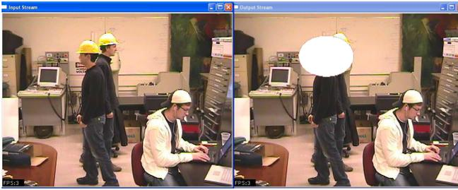
Fig. 4. Sample image frame input on left image, with output regions overlaid on right image. This sample illustrates tracking during a crossing, showing how the Particle Filter grows to accommodate both hats.
