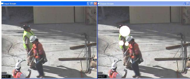
Fig. 6. Sample image frame input on left image, with output regions overlaid on right image. This sample illustrates how without Particle Filtering, partial occlusions segment the visual marker, resulting in multiple small ellipses.
