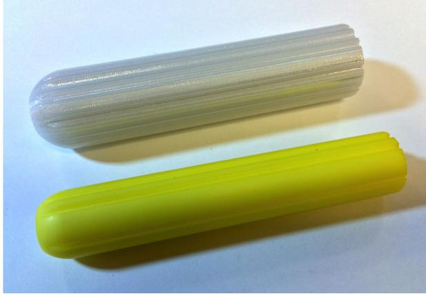
FIG. 1. 3D printing allows surgeons to customize the size and shape of brachytherapy applicators to improve treatment. Shown above is a 3D printed applicator made of PC-ISO (white). This applicator was designed to fit a patient with a very wide vaginal canal, which was too large for the largest commercial applicator of the same type at our clinic (yellow).
