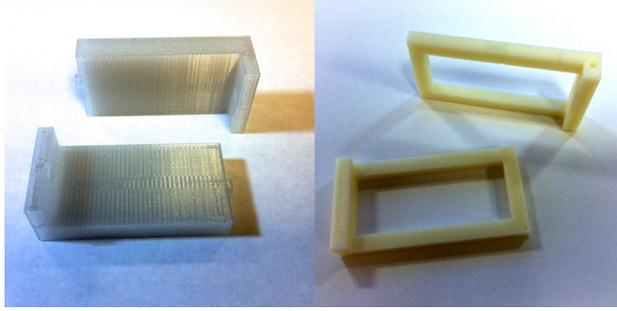
FIG. 2. A set of testing apparatus were designed and 3D printed for this study to measure the depth-dose curve for  $^{192}\text{Ir}$ . The apparatus held a piece of radiochromic film and an endobronchial brachytherapy catheter. The left picture shows testing blocks printed in PC-ISO, and the picture on the right shows control blocks used to suspend a piece of radiochromic film in water. The blocks were scanned in a helical CT to compute the Hounsfield unit distribution.
