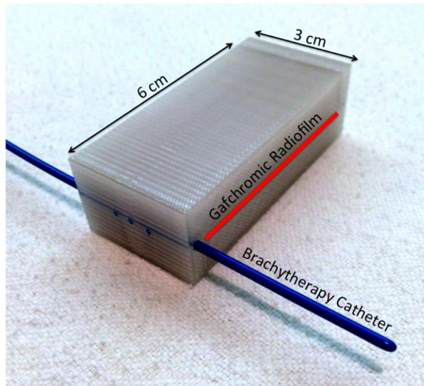
FIG. 3. A size 6 French endobronchial brachytherapy catheter was inserted into the block. The PC-ISO and control apparatus were suspended in water before the dose was delivered.
