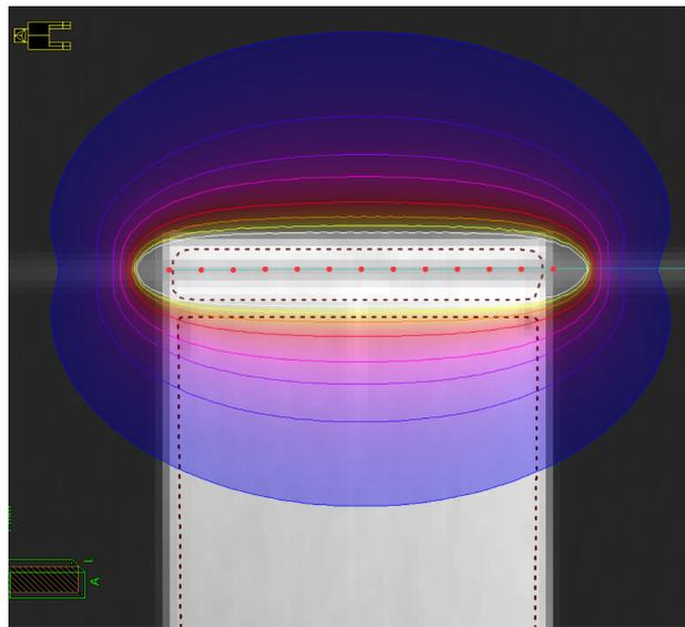
FIG. 4. A dose plan was computed in Oncentra to deliver 1500 cGy at 1 cm from the center of the catheter channel. The dwell positions and radial dose distribution for the radiochromic film study are shown above as seen on the planning system. The films were developed for 24 hours after exposure before they were scanned to find the dose-depth curve.
