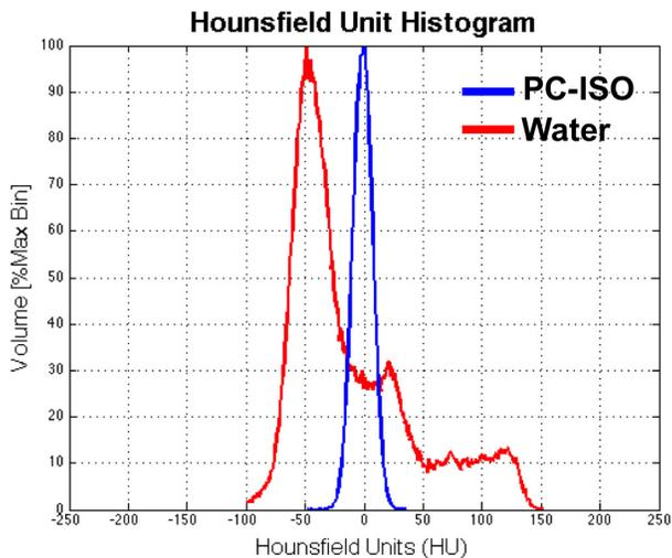
FIG. 5. Shown above is the distribution of Hounsfield units (HU) inside the PC-ISO apparatus. The mean was -1 HU for water and -10 HU for PC-ISO. This mean HU value is closer to water than air ( $\approx -1000$  HU) or bone ( $\approx 1000$  HU).
