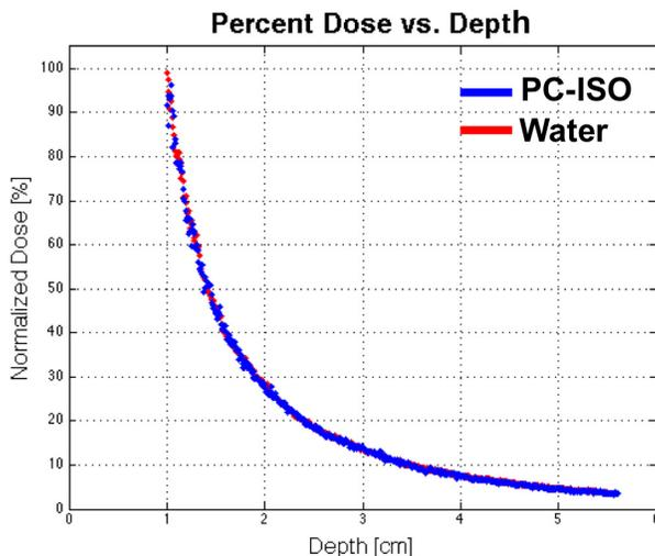
FIG. 6. The percent dose depth from the radiochromic film test for the testing apparatus (PC-ISO) and the control apparatus (water). The two curves were within 1% of each other between 1 cm and 6 cm, showing that the TG-43 planning system, which assumes a water medium, can be used as normal.
